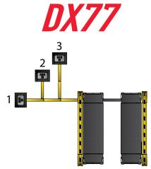
Manufacture provided 60" (standard length) air and hydraulic hoses allow three ergonomic, recommended power console placement options. Challenger Lifts new DX77 7,700 lb. capacity scissor lift was engineered with efficiency and productivity in mind. Our scissor lift can easily lift all makes and models (within rated capacity) with synchronized hydraulic system. Diamond plated flip-up approach ramps allows the platform to extend to accommodate longer wheelbase vehicles.
