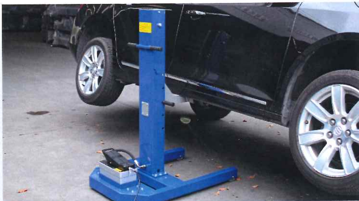
Lifting on the Underdoor
