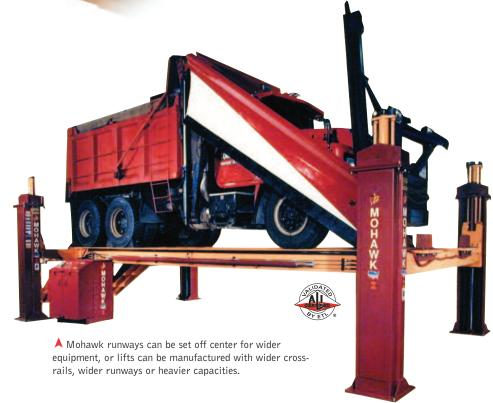
▲ Shallow angle approach ramps are 24" wide for easy drive on with the ability to accommodate a wide variety of vehicles (including low floor busses.) Shorter/longer or moveable ramps upon request.
