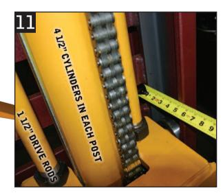
▲ Mohawk columns are made of 6" x 1" thick fork lift mast sections, with carriages riding on 4" sealed ball bearing rollers and raise via direct drive lifting rods.
