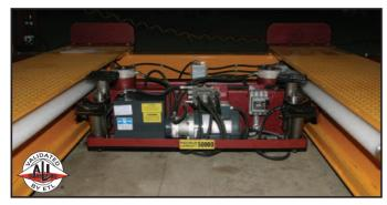
**Mohawk's RJ-50:** 50,000 lb. capacity rolling electric/hydraulic low profile jacks for "wheel free" tire and brake service. Jacks roll the full length of the runway, or use two jacks to raise the entire vehicle off of the runways. Mohawk's rolling jacks lock in place when loaded.
