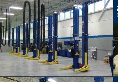
2 Posts lifts with lifting capacities of 10,000 lbs/11,000 lbs/12,000 lbs/15,000 lbs/20,000 lbs
