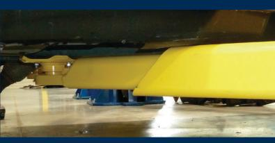
Adjustable 130" to 144" low ceiling lifts with lifting capacity of 9,000 lbs
