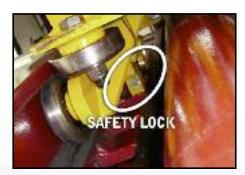
ALL position 1" thick mechanical locks on BOTH carriages engage the *full length* of travel.
