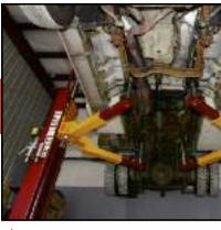
▲ Two post lifts offer FULL unobstructed ur for all repairs, take up minimal bay space hanging free for tire, brake or any other nece
