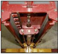
▲ Heavy duty column construction with dual cylinders, direct drive lifting rods (not cables) and stainless steel hydraulic lines (not rubber hoses) both of which will never wear.
